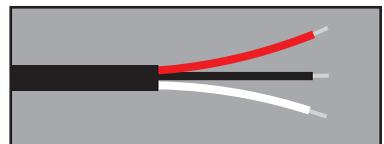
Red Wire (+12V DC) = Forward Projecting Trigger
