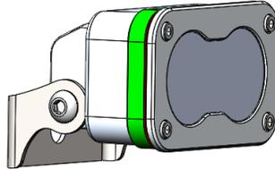
5. Using the 9/16" wrench and socket wrench, mount the light assemblies to the brackets from step 2. Slide reverse light bracket up or down until desired fitment is reached. Tighten the reverse bracket down with the 13mm socket wrench, and then tighten the rest of the hardware on the light assembly. Make sure to route the power chords away from any exhaust pipes and into the backside of the bumper.
