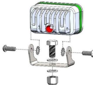
**\*Note: thread in 3/8" bolt before attaching light to bracket.**
