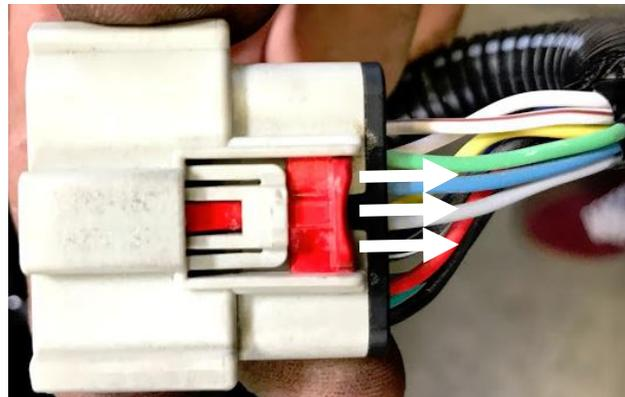
7. To disconnect the taillight plug, pull the red tab up until it appears as the picture on the right above. Now press the white detent in and pull the plug from the light.
