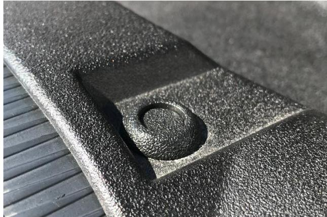
3. Now, it is important to remove each fastener individually, or else they will most likely be thrown in every direction while removing the panel. Removal of the fasteners can be completed by hand, or assisted by the use of a standard screwdriver. Once the fasteners are removed, the radiator cover can then be taken off of the vehicle.
