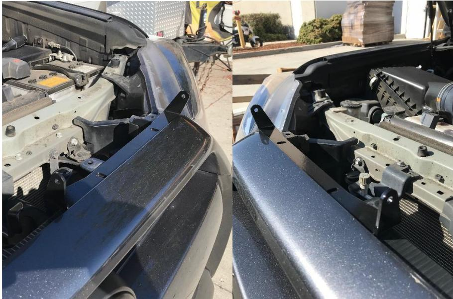
6. Now it is time to mount each light into a bracket. Using a 7/16" socket, tighten the provided 1/4" diameter bolt with washer through the bracket into the light housing. Make sure that the desired angle is set at this moment. The entire light/bracket assembly will have to be removed to make adjustments. Place the 5/16" bolts and accompanying washers through the bracket.
