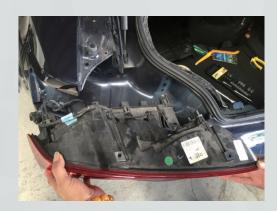
7. To release the stock wiring connector, pull the red lock out then press the center tabs beneath it to release the connector's latch.
