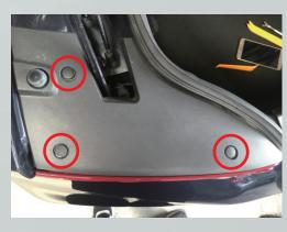
5. Remove the three (3) 8mm nuts holding the tail light to the vehicle.
