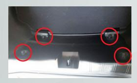
3. Remove the interior panel trim clips with a Y-shaped trim removal tool or carefully with a flathead screwdriver.
