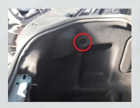
4. Remove the clips securing the trim panel on top of the tail lights. Remove the board and set aside.
