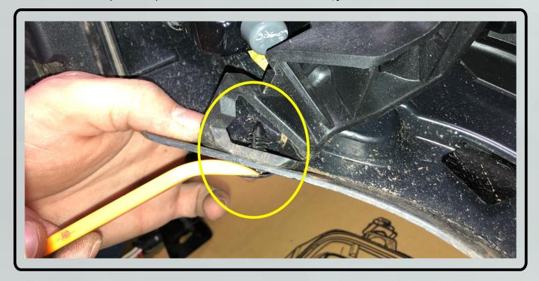
6. Remove the T25 Torx screw holding the side marker in place.
