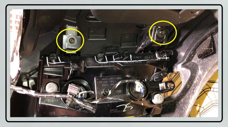
8. Unplug the small 2 pin connector for the OEM Amber sidemarker. It can then be removed by sliding it forward and away from the DRL/Fender.
