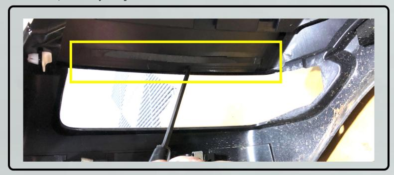
10. Remove the OEM wire harness for the stock DRL that runs to the back of the fender. There are a couple clips holding it in. Then re-route the harness for the new LED DRL back in the same place.
