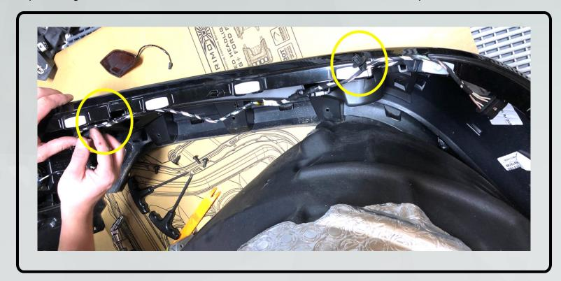
11. Re-install the new LED DRL in exact reverse order that was just used to remove the OEM assembly, starting with using the provided double-sided tape to replace the original. (not shown)
