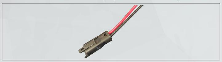
NOTE: On the premium edition there are only 5 of the 6 pins used, (Pin 3, the second ground, is gone). Pin 6 is the common ground. The Side marker is powered off pin 4 which is also the low output DRL. On the base model wiring Pin 1 is what powers the side marker. So for the premium models the side marker needs to be powered off pin 4 not pin 1. This would fix the issue with the side marker not working at all.
