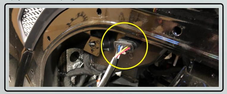
4. Unscrew the three T25 Torx screws on the bracket the bracket behind the OEM DRL.
