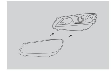
Place headlight housing in oven for seven (7) minutes at 270 Fahrenheit to soften the headlight sealant again.
