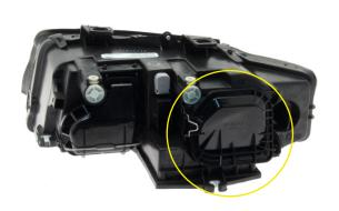
Remove the three nuts that secure the OEM projector. Install the Mini H1 projector in its place, and reinstall the OEM screws to retain the new projector.
