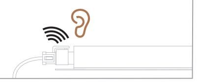
Do not mount ballast with connectors aimed upward!
