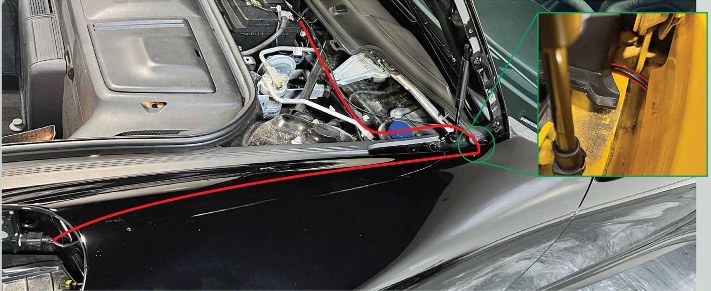
8. Route the passenger side DRL Harness as pictured below. Run it under the windshield cowl and into the inside of the fender. using a wire snake run it along the top channel on the inside of the fender.
