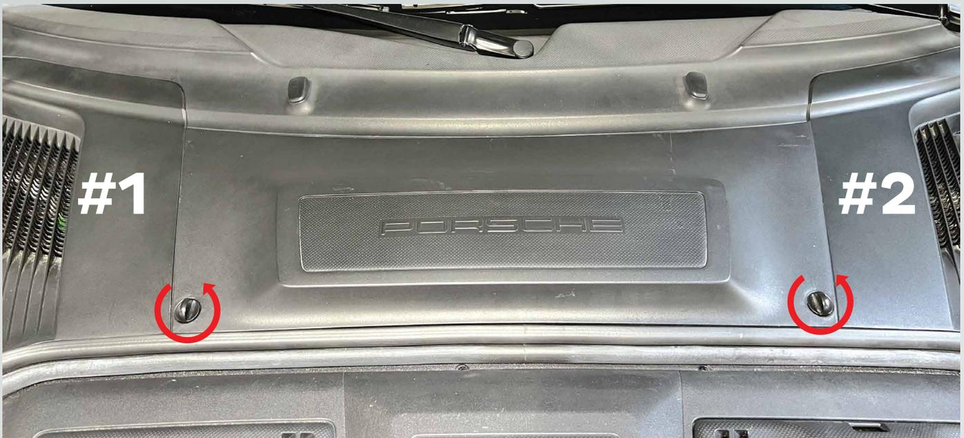
7. Locate the included DRL Harness, route the driver side of the DRL Harness as pictured below. Run it under the windshield cowl and into the inside of the fender. using a wire snake run it along the top channel on the inside of the fender.
