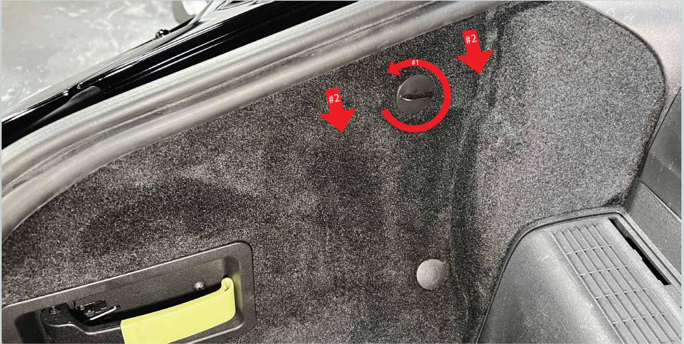
2. With the liner pulled back, remove this rubber plug. Do this by simply pulling it away from the sheet metal. Repeat steps #1, 2 on the other side of the car.
