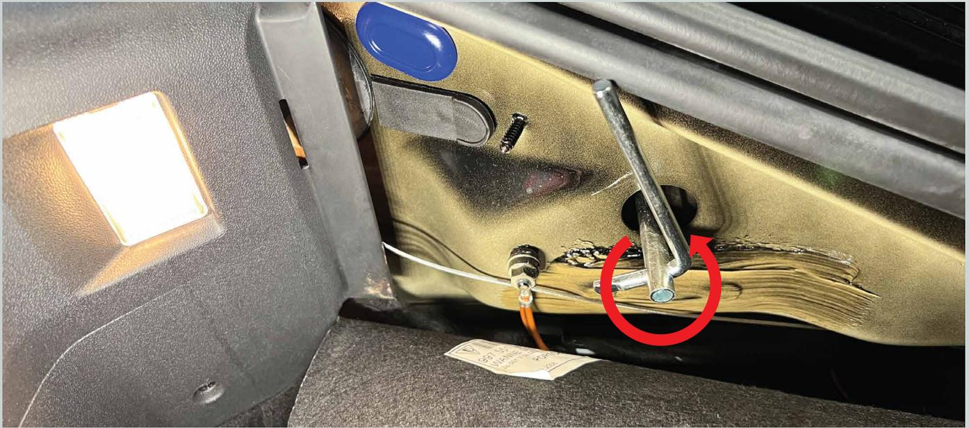
6. Remove the battery cover by rotating the two (2) plastic screw 90 degrees counter clockwise. Then simply pivot the front edge of the battery cover up and take the battery cover out of the car. Then remove the panels labeled #1, #2 in the picture. To remove them simply lift them up and out of the car.
