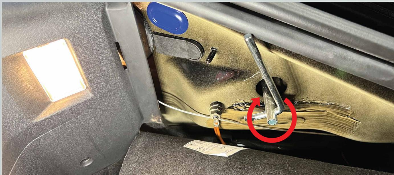
10. Transfer the headlight removal tool to the passenger side, grab your passenger side Morimoto headlight, bring it to the car and plug in the DRL harness. Next line up the guide pins on the sides of the headlight with the channels on the vehicle and slide the headlight into it's place. With one hand turn the tool counter clockwise while pressing the headlight into the fender with the other hand. Carefully turn the tool til you hear a pop sound.
