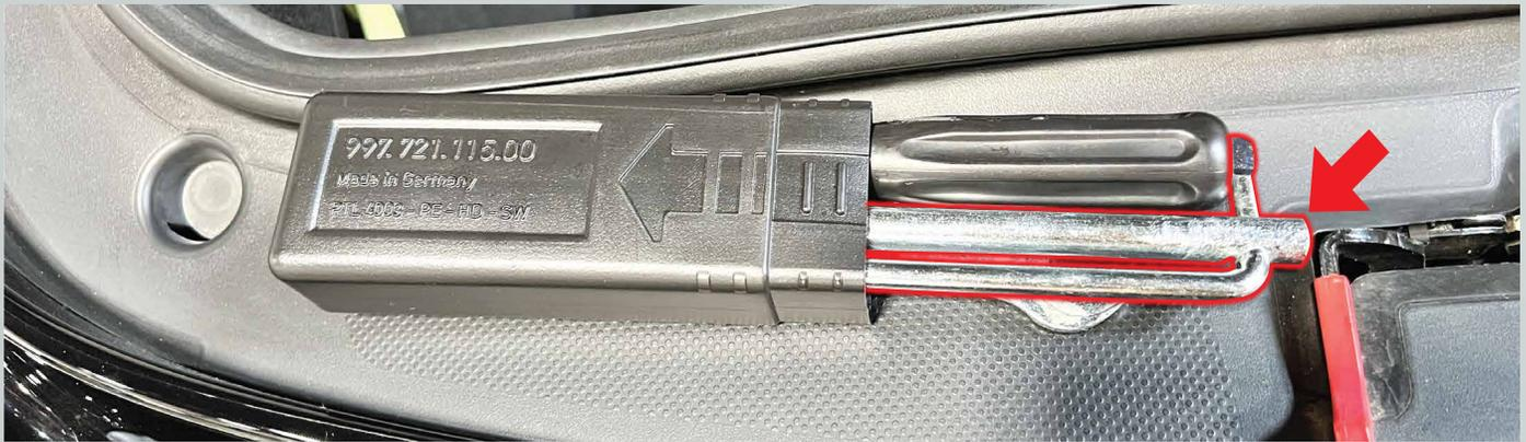
4. Starting on the passenger headlight, insert the headlight removal tool into the hole that had the rubber plug. Note that inserting the headlight removal tool might take a few tries for it to seat on the bolt head. With the tool correctly seated, rotate the tool clockwise approximately 90 degrees til the headlight pops forward. Then simply slide the headlight forward away from the car and set the headlight to the side.
