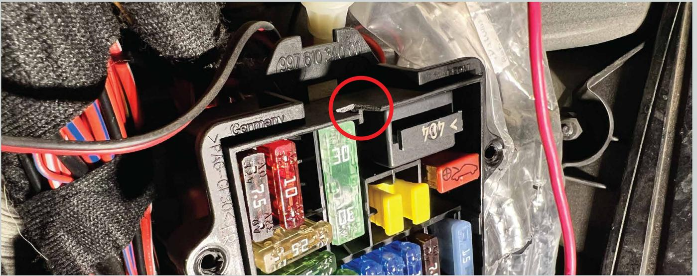
15. Remove fuse C2 7.5 A fuse and plug in the Fuse Tap Harness in place of that fuse. Reassemble the kick panel.
