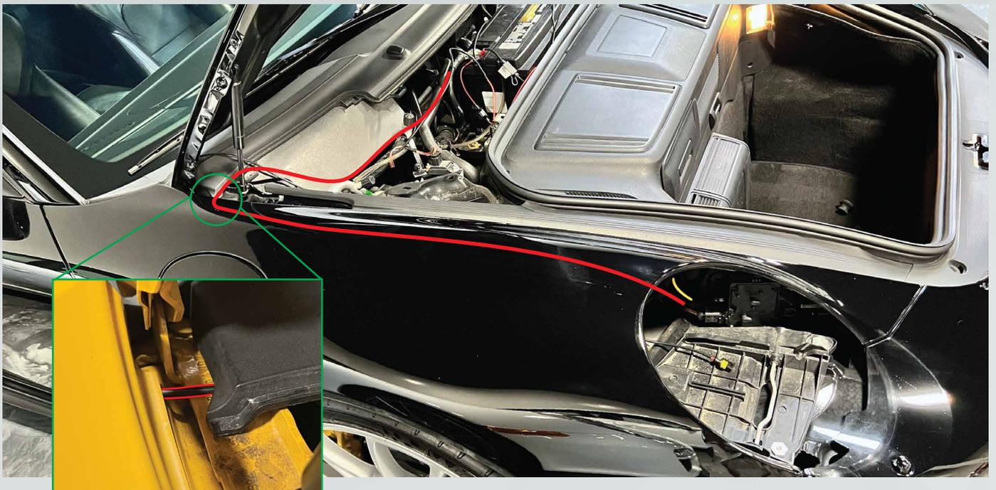
9. With the headlight removal tool still inserted on the driver side, grab your driver side Morimoto headlight, bring it to the car and plug in the DRL harness. Next line up the guide pins on the sides of the headlight with the channels on the vehicle and slide the headlight into it's place. With one hand turn the tool clockwise while pressing the headlight into the fender with the other hand. Carefully turn the tool til you hear a pop sound.
