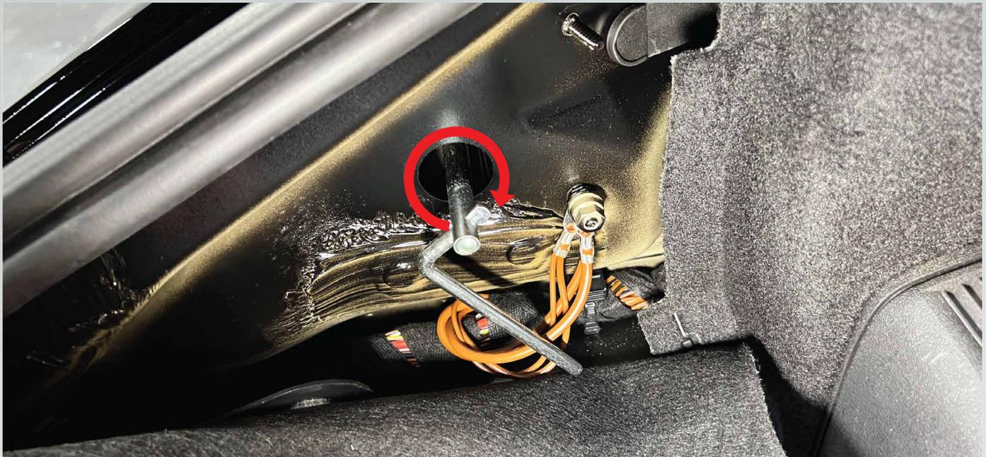
5. On the driver side headlight, insert the headlight removal tool. Rotate the tool counter clockwise about 90 degrees til the headlight pops forward. Then simply slide the headlight forward away from the car and set the headlight to the side.
