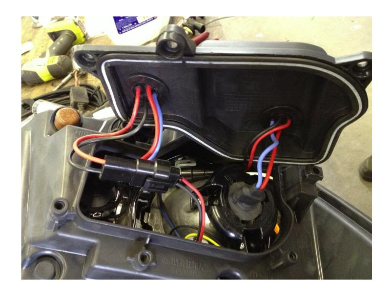
Once you have all the wires through the dust cover you can put the black plastic 2-pin connector back together with the red and black wires and re-secure the dust cover onto the headlight.
