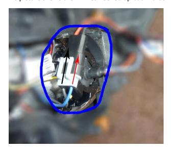
You can see in this picture the blue wire on the truck (the factory + wire) is connected to the black HID wire which is – ground. This connection needs to be flipped around, either right here, or where it plugs into the ballast. You can either cut and splice the wiring so it flips them around, you can de-pin the black connector and flip the wires around or you can just plug the connector in backwards to make sure the positive and negative wires match up.
