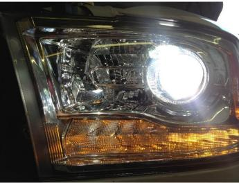
These new headlights use what is called a 9012 or 9012LL halogen bulb and although it looks like a standard halogen incandescent bulb, technically it is called "HIR" or "Halogen Infra-Red". Even though it's a new type of halogen bulb, most Ram owners still say they are terrible and should be brighter. Doing an HID conversion kit in the new Ram trucks is safe, doesn't void warranty, and is how the truck should have come from the factory, as long as you use the right parts!
