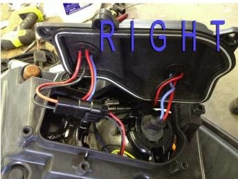
The HID bulb has 4 wires attached to it within the harness. A red and blue set of wires and a red and black set of wires. The red and black wires connect to the factory headlight wiring. The red and blue wires connect to the new HID ballast:
